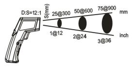
3. Field of view: Be sure the target area is larger than the unit's spot size. The smaller the target get, the closer the measured distance. For precise measuring, make sure the target is at least twice as large as the spot size.
