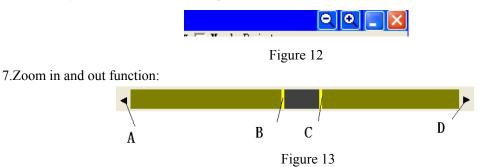
7.1 When the data set number is more than 200 groups, enlarged curves can be displayed through double-click the curve of Figure 13.
